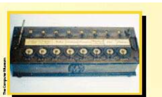
1642-1643 Blaise Pascal creates a gear-driven adding machine called the "Pascaline," the first mechanical adding machine.
